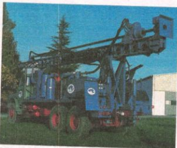
The TD 500 truck-mounted drill.
