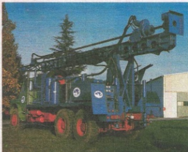
The TD 500 truck-mounted drill.
