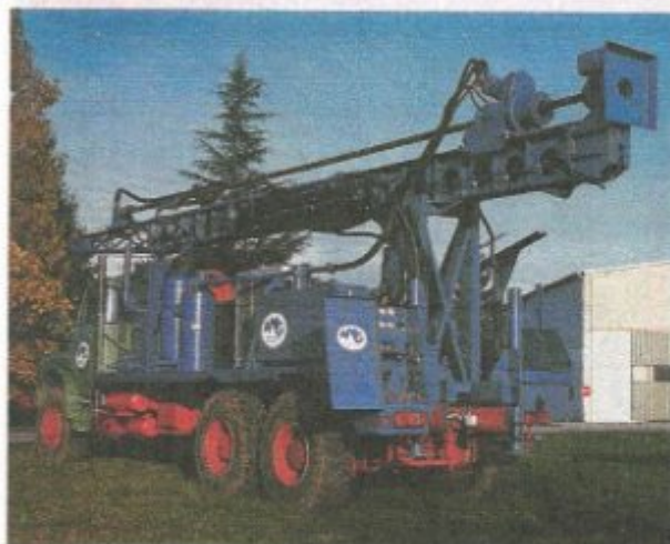
The TD 500 truck-mounted drill.
