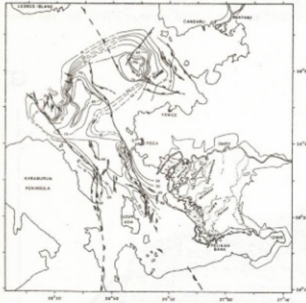
Fig. 16. Isopach map of Depositional Sequence 2 as related to sedimentation from Gediz river, showing sediment thickness in milliseconds two-way travel time. Heavy lines are faults with ticks on downthrown side. Acoustic source: air-gun.
