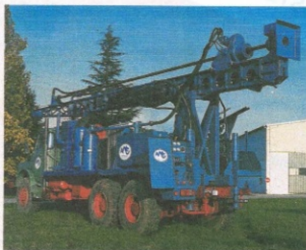
The TD 500 truck-mounted drill.
